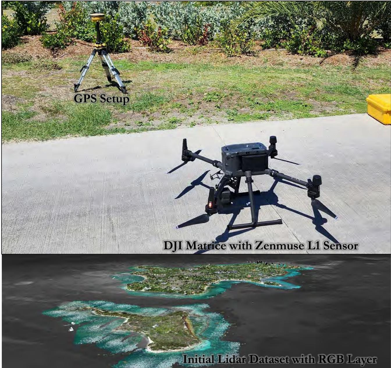
**Figure 2.1 Apparatus used for the LiDAR survey and initial results for the islands surveyed.**
