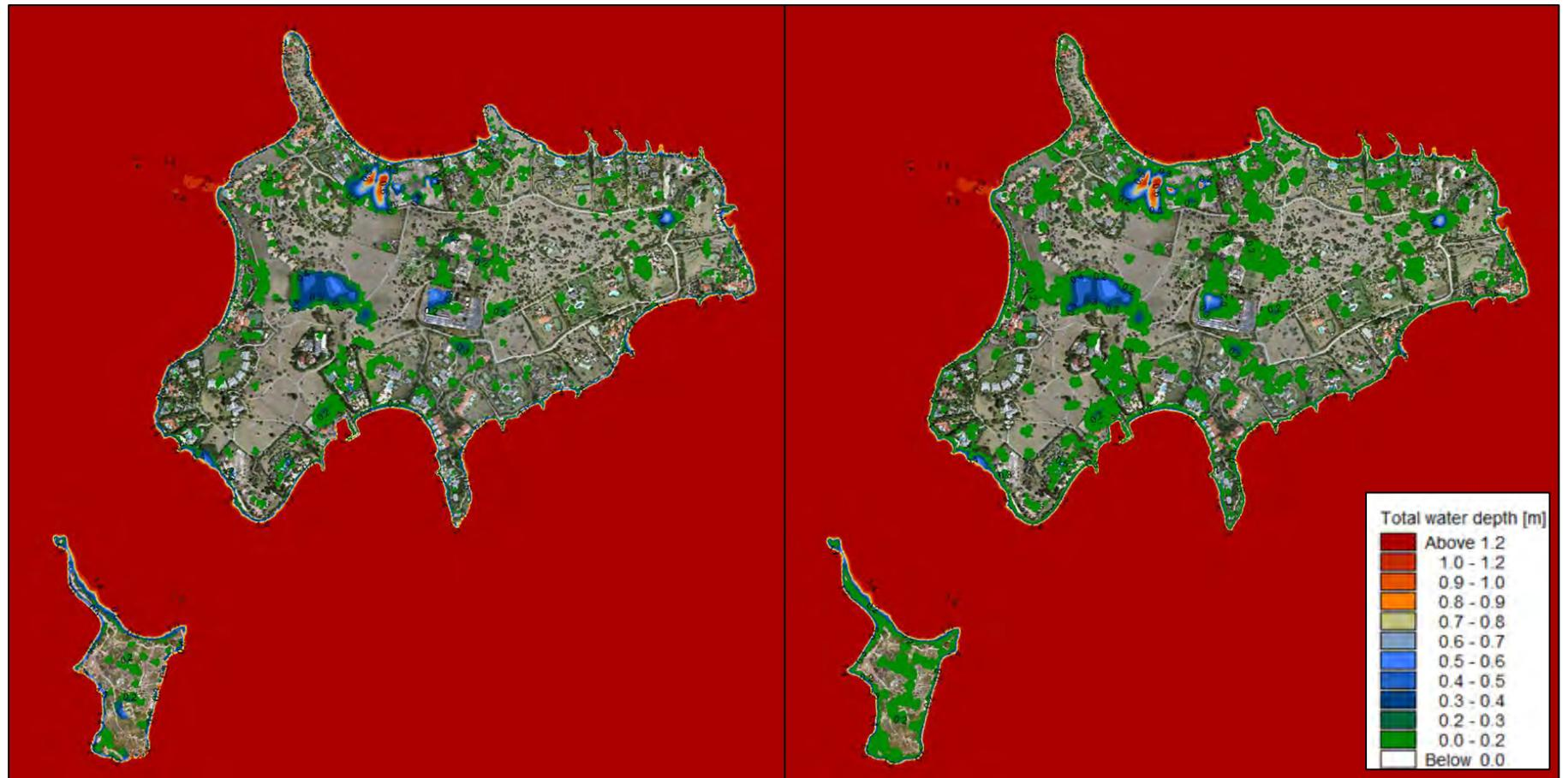
Figure 7.1 Flooding (ponding) simulation results from the 50-year rainfall event (left) and from 100-year rainfall event (right).
