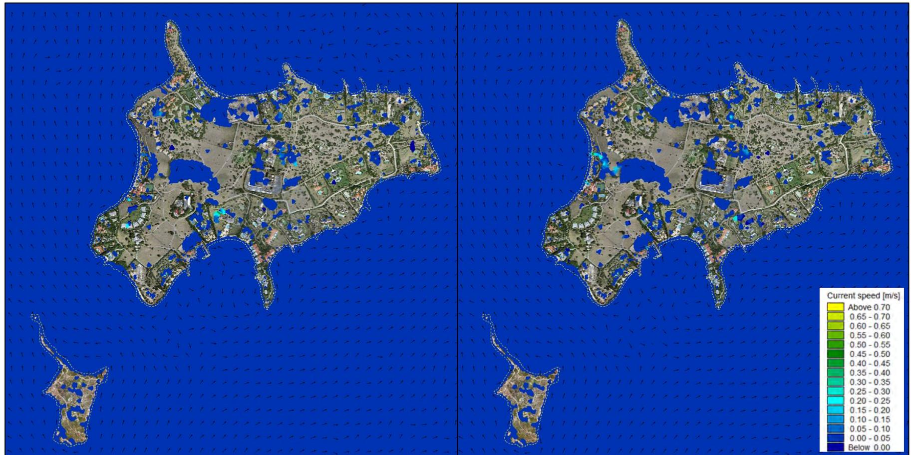
Figure 7.2 Current speed simulation results from the 50-year rainfall event (left) and from 100-year rainfall event (right).
